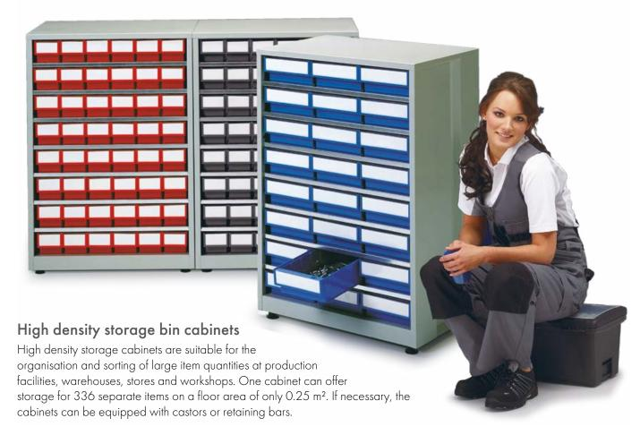
This product includes a frame, bins and labels with protective shields. Backstops hold the bins when fully extended. Adjustable feet are provided for fine levelling of the cabinet on uneven surfaces. The load capacity of a cabinet is 240 kg, and that of a single shelf is 30 kg. The frame is made of grey powder-coated steel (RAL 7035). Profiled ends and a welded steel construction contribute to the general robustness of the frame. Details on the shelf bins can be found on pages 12 and 13.
